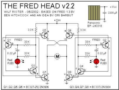
The main differences in Dangerbot! are the solar panel and power storage capacitor. Other than that, he's identical to this schematic. For a very technical description of this circuit, contact me and I'll send it to you. It involves learning about several previous incarnations of this circuit and a firm grasp on the operations of analog circuits. But... I can simply say to watch the FLED "eyes" to see when its about to "pop". This may
